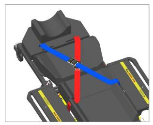
The head belts are mounted crosswise, always joining the upper and lower parts with the same colour.
