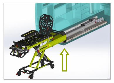
Once the stretcher is oriented on the side profiles, push the stretcher until it reaches the stop of the front wheels.
