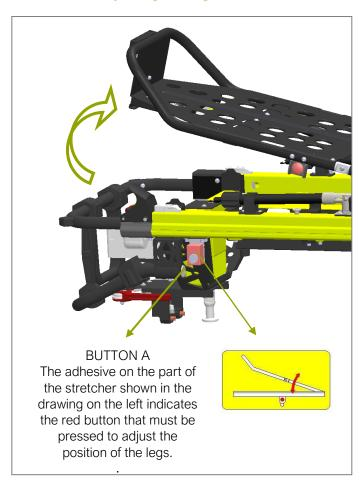
The required inclination of the leg rest can be obtained by pressing button A and moving the leg rest manually. Once the correct inclination has been reached, release button A to automatically lock the leg rest.
