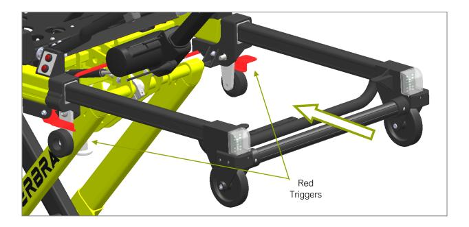
The head frame has a mechanical stop in the intermediate position (2090 mm long), one in the folded position (1723 mm) and one in the extended position (2210 mm). When the travel of the head frame reaches each of these three positions, the red lever "clicks" back into its original position.
