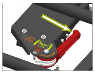
In the event of a malfunction of the hydraulic system, the stretcher can be operated manually. For the following procedure, it is essential that the stretcher is handled by two operators. With the stretcher in the unfolded position, pull the red trigger located next to the battery at the rear of the stretcher. The stretcher will lower to the lower stop and remain in this position.
