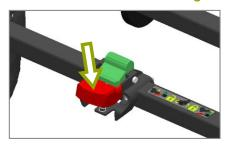
Pressing the red centre lever allows the wheels to turn freely. Pressing the green rear lever blocks the free rotation of the wheels
