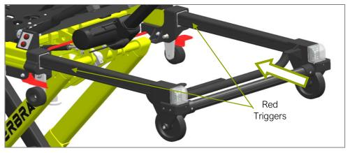
The head frame has a mechanical stop in the intermediate position (2090 mm long), one in the folded position (1723 mm) and one in the extended position (2210 mm). When the travel of the head frame reaches each
