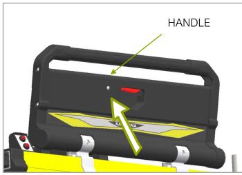
movement from the horizontal position to the 90° position is carried out manually. Once the desired position is reached, the position of the railing is automatically fixed.
