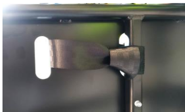
A: The straps of the chest-belts are threaded through the slot and tied around the crosspiece using the opening around it, as shown above.
